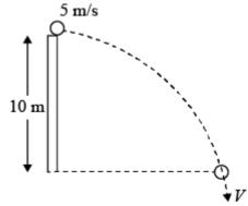
$$egin{aligned} v &= \sqrt{u^2 + 2gh} \ &= \sqrt{25 + 2 imes 10 imes 10} \ &= \sqrt{225} = 15 ext{ m/s} \end{aligned}$$
