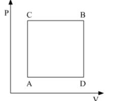
When path ACB is used 60 J of heat flows into the system and 30 J of work is done by the system. If path ADB is used work done by the system is 10 J. The heat Flow into the system in path ADB is: JEE 2019
