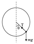
At any  $\theta$  :  $T - mg \cos \theta = \frac{mv^2}{R}$   $\Rightarrow T = mg \cos \theta + \frac{mv^2}{R}$ Since *v* is constant,  $\Rightarrow T$  will be minimum when  $\cos \theta$  is minimum.  $\Rightarrow \theta = 180^{\circ}$  corresponds to  $T_{\text{minimum}}$ .
