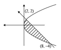
The required area= $\int_{-4}^{2} \left(4 - y - \frac{y^2}{2}\right) dy$ = $\left[4y - \frac{y^2}{2} - \frac{y^3}{6}\right]_{-4}^{2}$ = 18 square units
