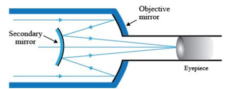
Telescopes with mirror objectives are called reflecting telescopes. A reflecting telescope is also called a reflector. The convex secondary mirror to focus the incident light, which now passes through a hole in the objective primary mirror, which is shown in the above diagram.
