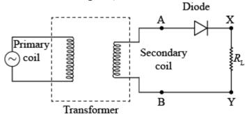
In the positive half cycle of a.c., the voltage at A is positive, the diode is forward biased and it conducts current.
